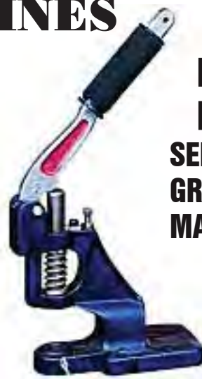
LOAD - Top Die holds grommet firmly.
